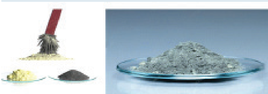
Figure 2.9 Separating iron from a mixture of iron and sulfur
