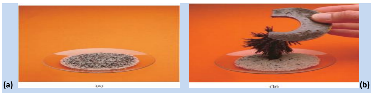
Figure 2.16 (a) the mixture contains iron fillings and sand. (b) A magnet separates the iron fillings from the mixtures.
